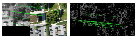
(a) Failed registration using SURF.
