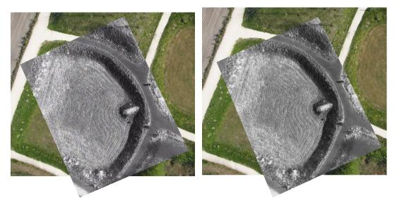
(c) Registered after homography of raw (dis- (d) Registered after homography of undistorted) images. torted images.
