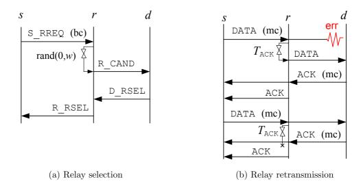
Figure 5.1: Message flow for periodic and adaptive relay selection (a) and relay operation after it is selected (b). Here and later in the text, *bc* and *mc* stand for a broadcast and a multicast transmission, respectively.
