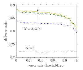
(a) Total delivery ratio with adaptive relay selection as a function of the error rate threshold  $\varepsilon_a$  over a window  $W_a$  of recently transmitted DATA packets.
