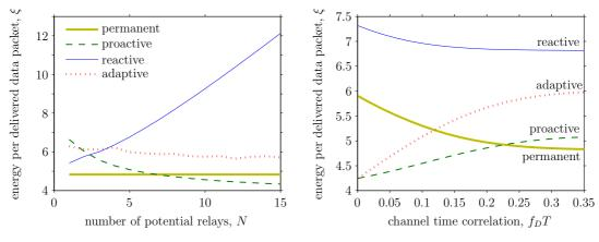
(a) Energy efficiency versus number of nodes; (i.i.d. channels.
