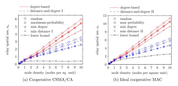
Figure 3.11: Expected relay spatial use  $a_r$  versus node density in the network for different combinations of utility and selection functions; contention window size w = 5.
