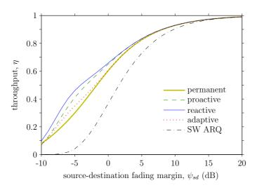
Figure 4.8: Throughput  $\eta$  as a function of source-destination fading margin  $\psi_{sd}$ . Number of potential relays N = 5, channel time correlation  $f_D T = 0.1$ , selection overhead sel = 0.
