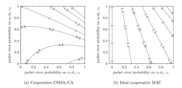
Figure 3.8: Ratio of overall network throughput with and without cooperation,  $\eta_{\rm co}/\eta$ , as a function of packet error rates  $\varepsilon_1$  and  $\varepsilon_2$  in the non-symmetrical network scenario;  $p_{R_1} = 0$ ,  $p_1 = p_2 = 0.75$ .
