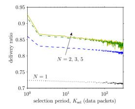
(a) Total delivery ratio with periodic relay selection as a function of relay update interval.
