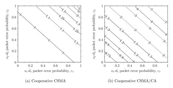
Figure 3.6: Ratio of overall network throughput with and without cooperation,  $\eta_{\rm co}/\eta$ , as a function of packet error rates  $\varepsilon_1$  and  $\varepsilon_2$  in the symmetrical network scenario;  $p_1 = p_2 = 0.75$ ,  $p_{R_1} = p_{R_2} = 0$ .
