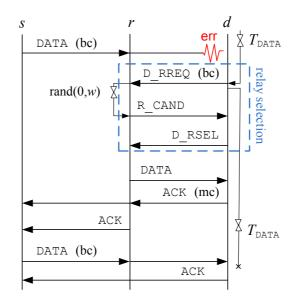
Figure 5.2: Message flow for cooperative ARQ with reactive relay selection.
