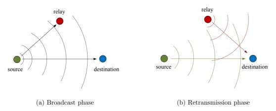
Figure 2.1: Concept of a relay channel.
