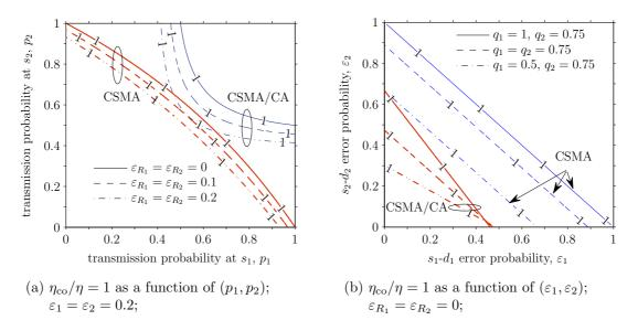
Figure 3.7: Equal overall throughput with and without cooperation,  $\eta_{\rm co}/\eta = 1$ , in the symmetrical network scenario.
