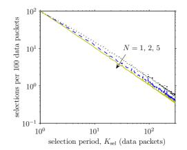
(b) Number of selections per sample with 100 packets as a function of relay update interval.
