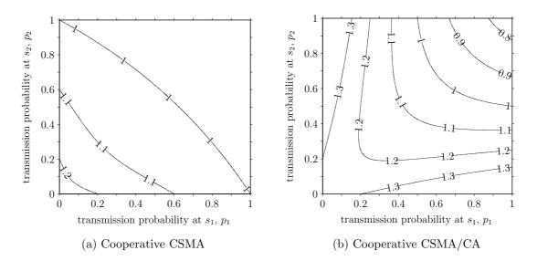
Figure 3.5: Ratio of overall network throughput with cooperation to that without cooperation,  $\eta_{co}/\eta$ , as a function of transmission loads  $p_1$  and  $p_2$  in the symmetrical network scenario;  $\varepsilon_1 = \varepsilon_2 = 0.2$ ,  $p_{R_1} = p_{R_2} = 0$ .
