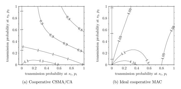
Figure 3.9: Ratio of overall network throughput with and without cooperation,  $\eta_{\rm co}/\eta$ , as a function of transmission loads  $p_1$  and  $p_2$  in the non-symmetrical network scenario;  $\varepsilon_1 = \varepsilon_2 = 0.2$ ,  $\varepsilon_{R_1} = 0$ .
