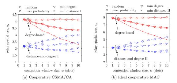
Figure 3.12: Expected relay spatial use  $a_r$  versus contention window size w for different combinations of utility and selection functions; node density is seven nodes per sq. unit.
