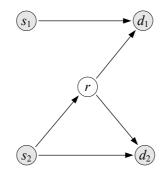
Figure 2.4: Interference at  $d_2$  introduce by the cooperative relay.
