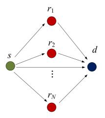
Figure 2.3: Use of multiple relays to assist s-d transmissions.
