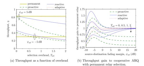
Figure 4.10: Impact of selection overhead on throughput; N = 5,  $f_D T = 0.1$ .
