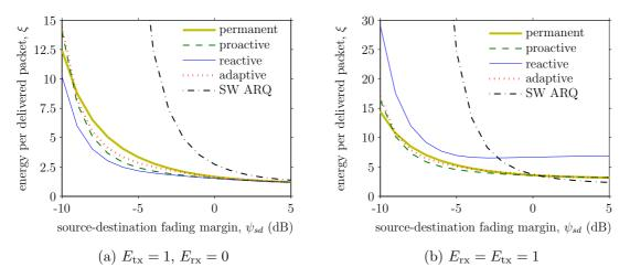
Figure 4.12: Expected energy per delivered packet  $\xi$  over source-destination fading margin  $\psi_{sd}$ ; N = 5,  $f_D T = 0.1$ .
