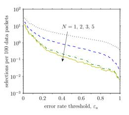
(b) Number of triggered relay selections per 100 transmitted DATA packets.
