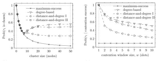
(a) Probability that  $r_1$  is chosen versus the number of nodes in the cluster; w = 5.
