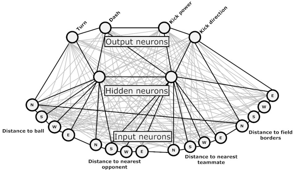
Figure 7.1: A possible wiring of the neural network showing the groups of inputs, outputs and hidden neurons. Connections with stronger weight are indicated with bold lines while ones with lower weight are colored with grey.
