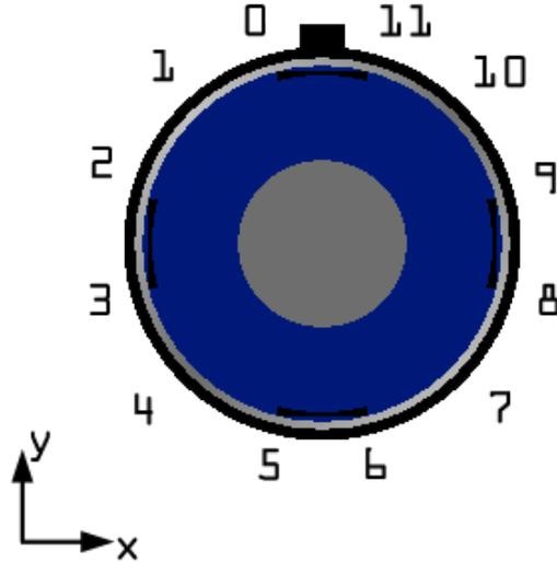
Figure 6.1: LED arrangement on the robot's body, as seen from top
