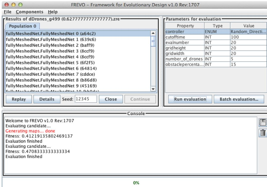
Figure 4.8: FREVO in evaluation mode. Left: list of candidates, right: configurable parameters
