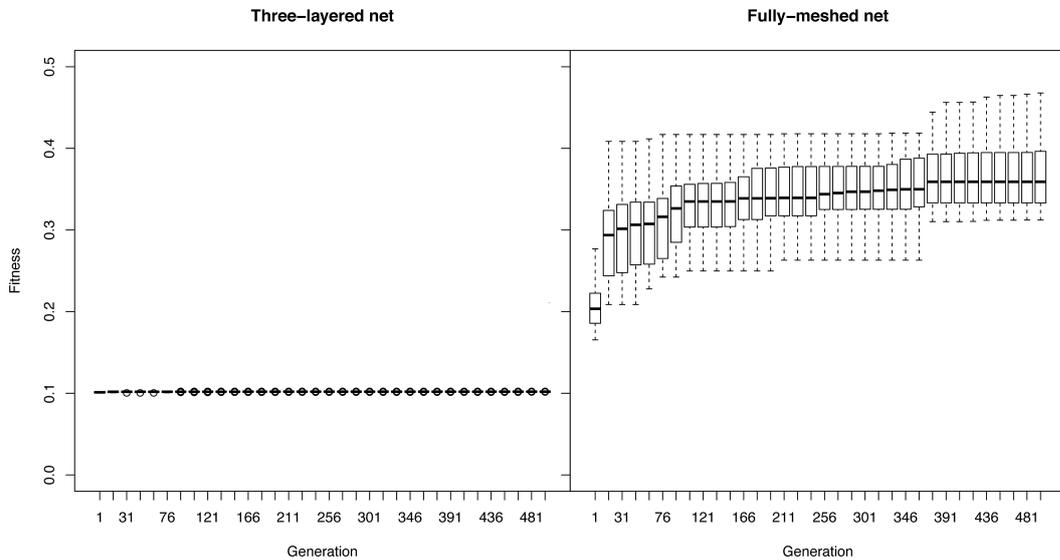
Figure 4.5: Fitness development vs. number of generations with different neural networks. Optimization method: *NNGA*, obstacle percentage: 0%. The *Fully-meshed net* clearly outperforms the *Three-layered net* in every generation.
