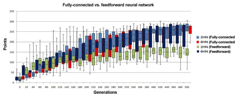
Figure 7.8: Box-and-whisker diagram of the repeated evaluation of fully connected vs. feedforward ANN with Cartesian interface
