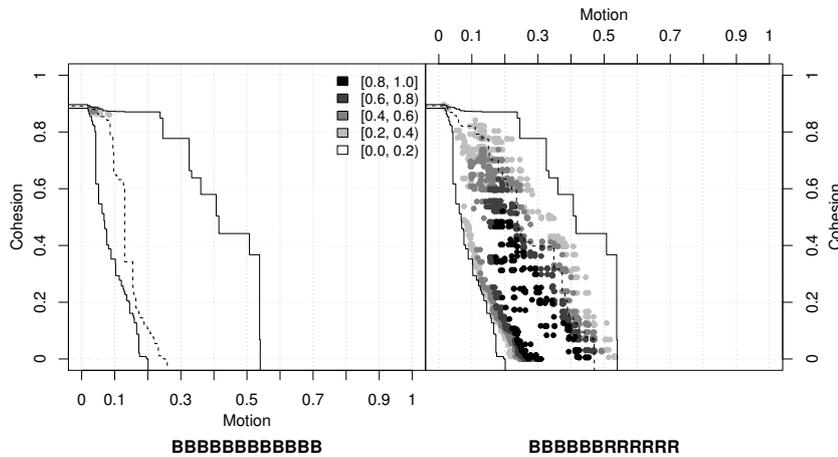
Figure 6.4: Comparison between the uniform configuration (BBBBBBBBBBBB) and a left-right configuration featuring an equivalent number of LEDs on (BBBBBBRRRRRR)
