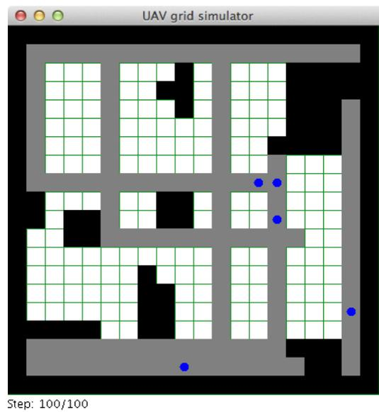
Figure 4.9: UAV example project visualization with 5 drones and 15% obstacles. Black cells are blocked, while grey ones are covered. The blue dots indicate the position of the drones.
