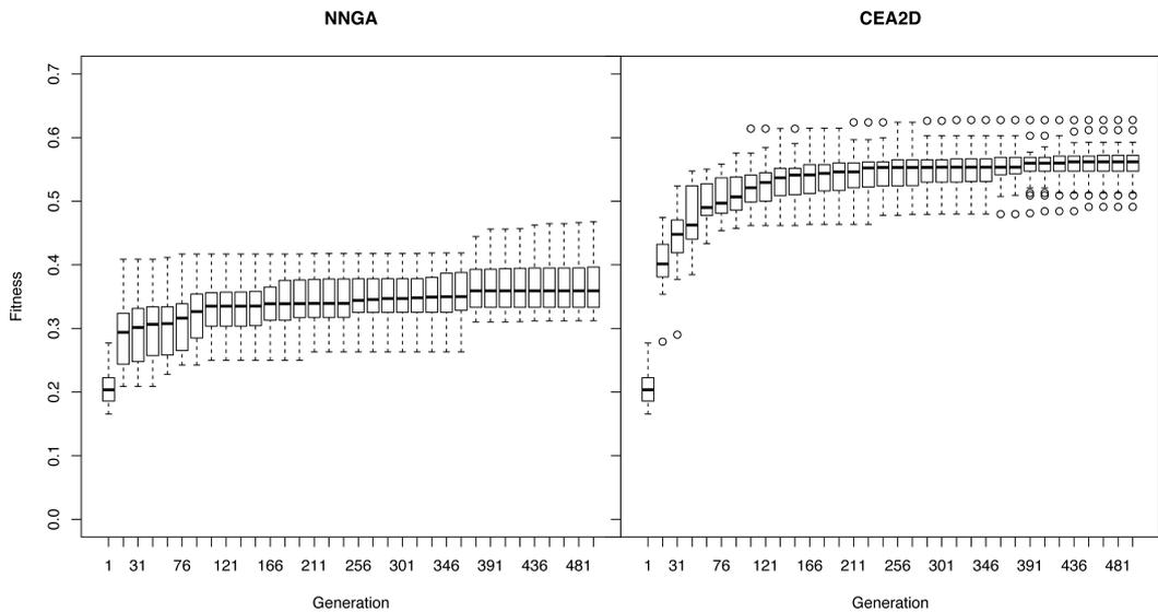
Figure 4.6: Fitness development vs. number of generations with different optimization methods. Representation: *Fully-meshed net*, obstacle percentage: 15%. *CEA2D* outperforms *NNGA* in almost every generation.
