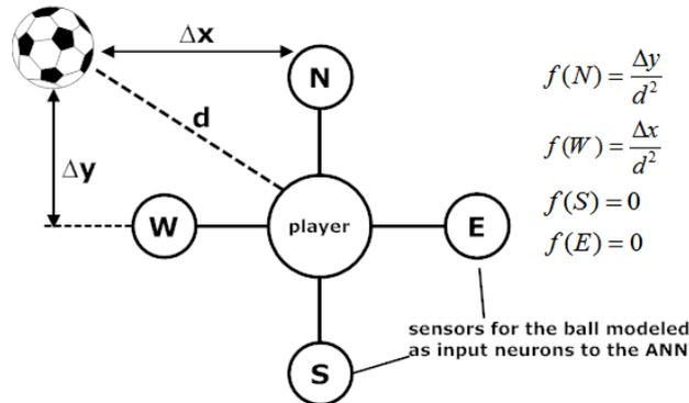
Figure 7.2: A group of input neurons detecting the ball
